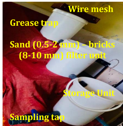
(b) Waste water treatment setup
